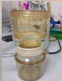
Filtration unit used in water testing.
